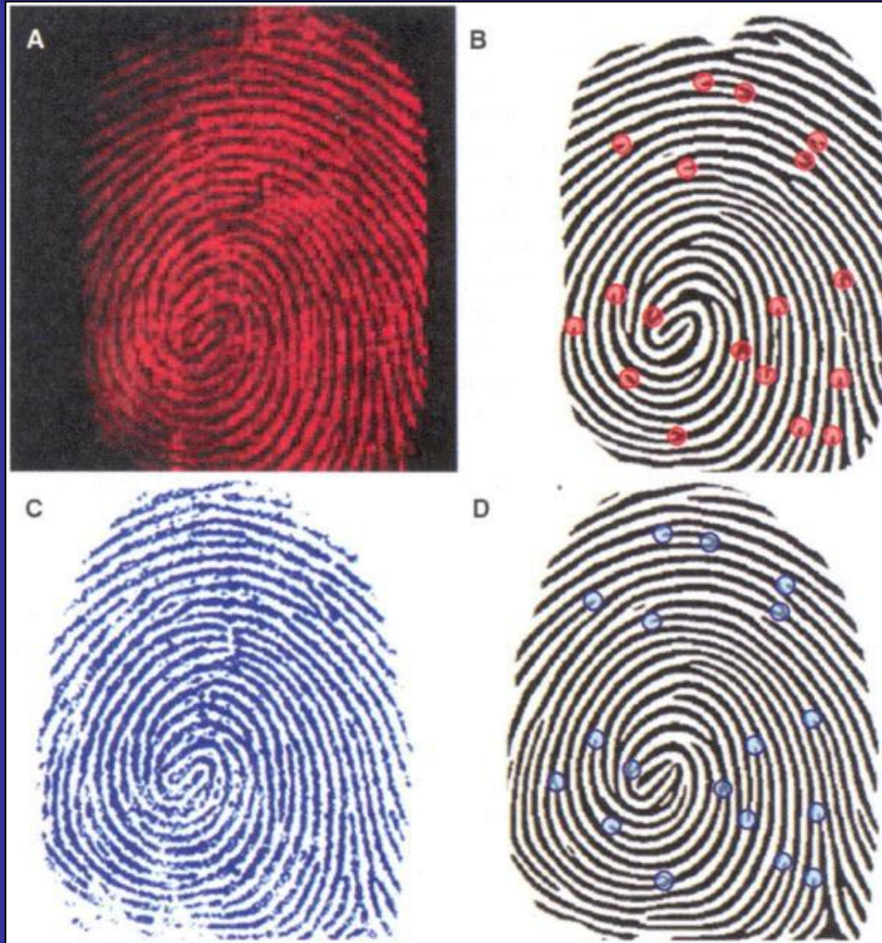
Fig. 1 . (A) DESI image of distribution of cocaine on a LFP blotted on glass. (B) Computer-generated fingerprint from DESI image. (C) Ink fingerprint blotted on paper and optically scanned. (D) Computer-generated fingerprint from optical image. Some of the automatically detected points of interest (minutiae) are represented by dots in (B) and (D).
