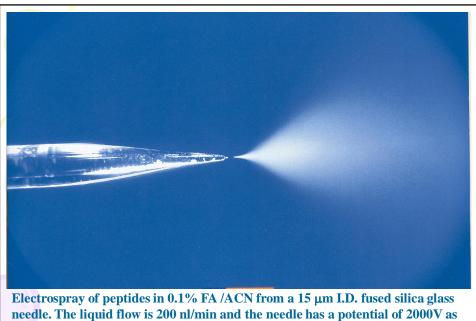
compared to the cone inlet of the mass spectrometer.
